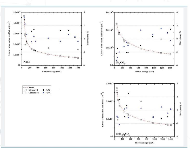
Figure 3: The variation of the XCOM, calculated and measured linear attenuation coefficient of the various samples of NaCl,  $Na_2CO_3$  and  $(NH_4)_2SO_4$  and their discrepancies as a function of the photon energy.
