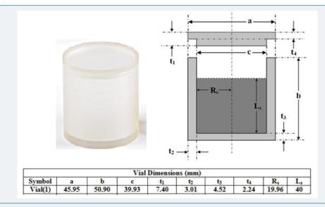
Figure 2: The Plexiglas sample vial with cross sectional drawing and dimensions.
