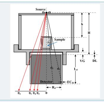
Figure 1: Source and detector arrangement in terms of the photon length throught the sample and the detector.
