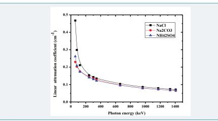
Figure 4: The variation of the calculated linear attenuation coefficient of the various samples of NaCl, Na,CO, and (NH<sub>4</sub>)<sub>2</sub>SO<sub>4</sub> as a function of the photon energy.
