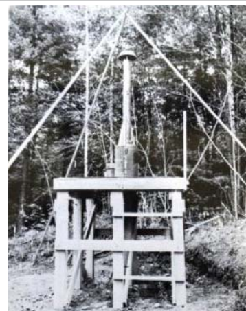
Figure 2: The 10,000-Ci ^{137}\text{Cs} radiation source in position in site 1.
